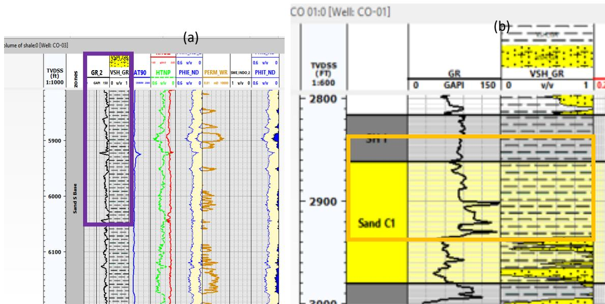
Fig. 6: This is a Shale unit with blocky shape as indicated in the blue rectangle (a), while (b) is a sandy shale (shale with small sandstone/ mud stone) is recognised by its serrated shape.
