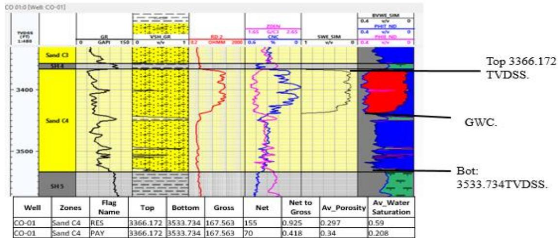
**Fig. 9:** Sand C4 is a good reservoir sand from the gamma ray log, resistivity value indicates that there is fluid, using neutron –density crossover indicates that there is gas. The water saturation and porosity (both total and effective) value is good.
