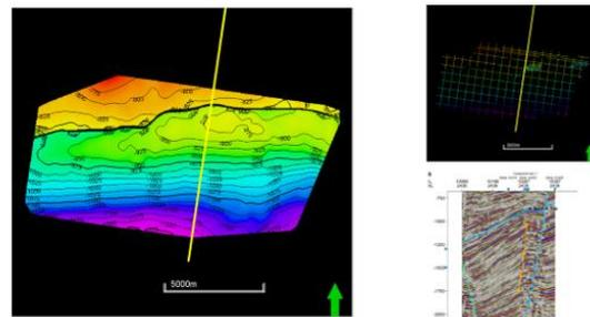
**Fig.s 11: Horizon interpretation and time map generated from sand C2 reservoir of Maboro-Field.**
