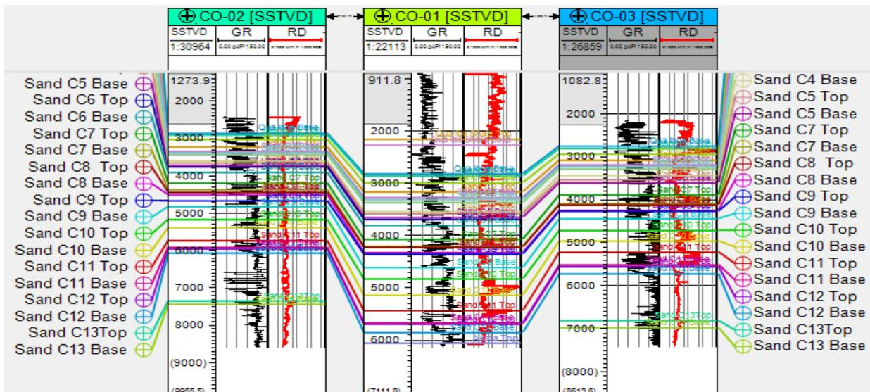
Fig. 7: well log correlation in Maboro-Field which shows that the reservoirs are continuous.
