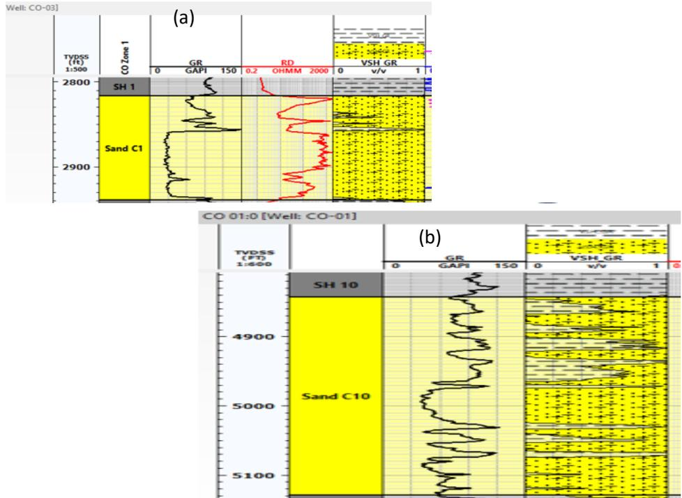
Fig. 5: shows Clean sandstone reservoir with low gamma ray, cylindrical shape (a) while (b) is sandstone reservoir with thinly bedded shale and has bell shape known as sandy shale/ silt stone.
