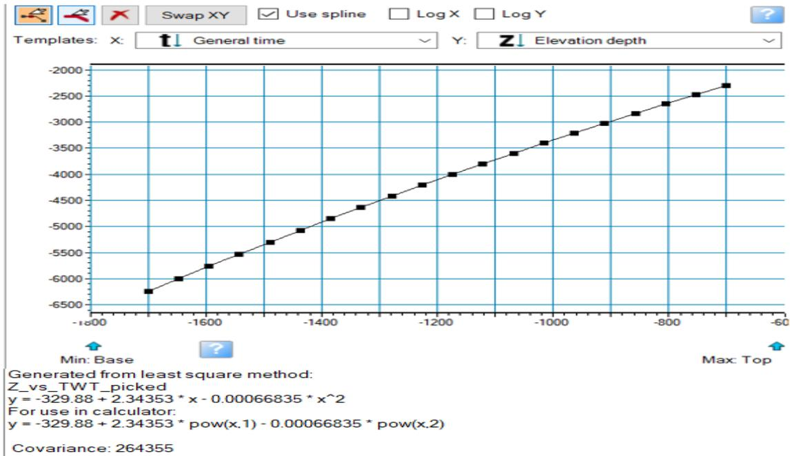
Fig. 12: Depth conversion model, the two-way time used to convert time map to depth
