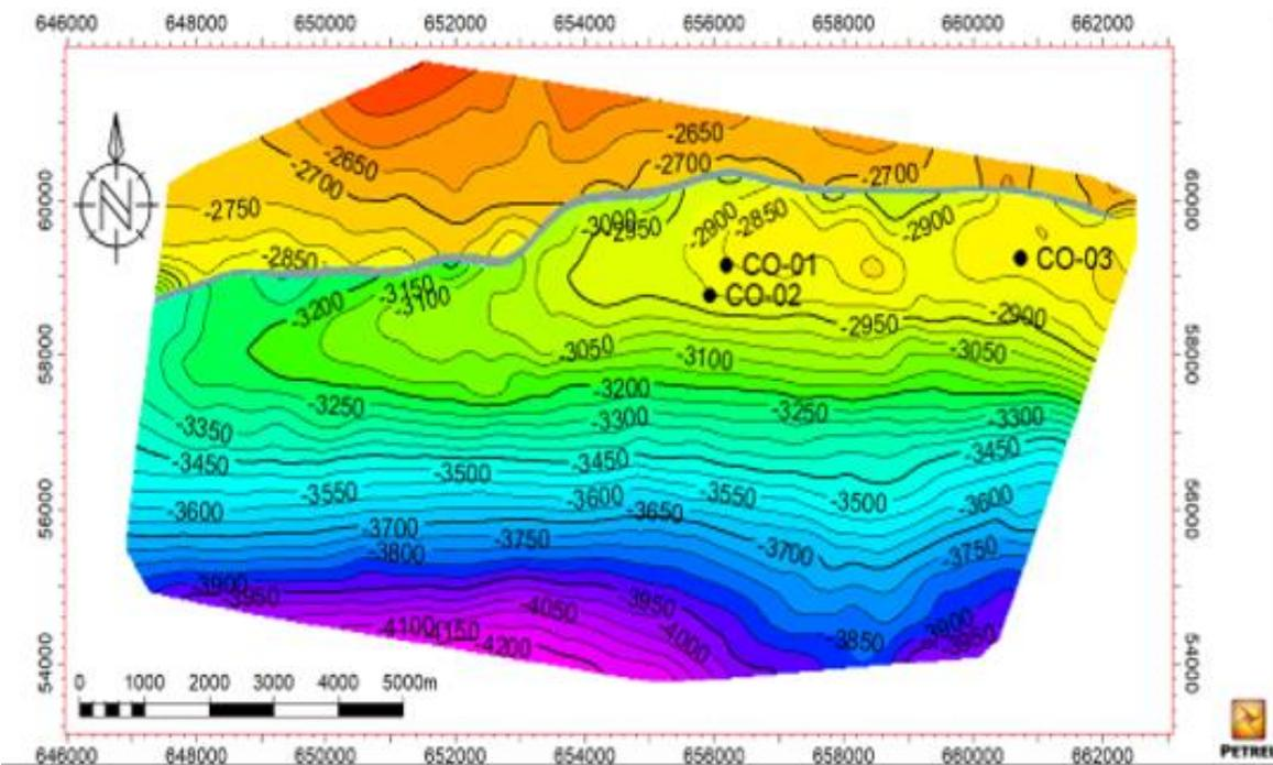
Fig. 13: Generated depth map from sand C2-reservoir of Maboro -Field.
