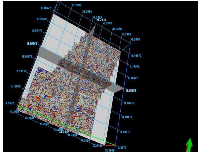
**Fig. 9: 3-D seismic section showing Area extent (inline, crossline and time-slice) covered by Maboro-Field 99.9 K**
