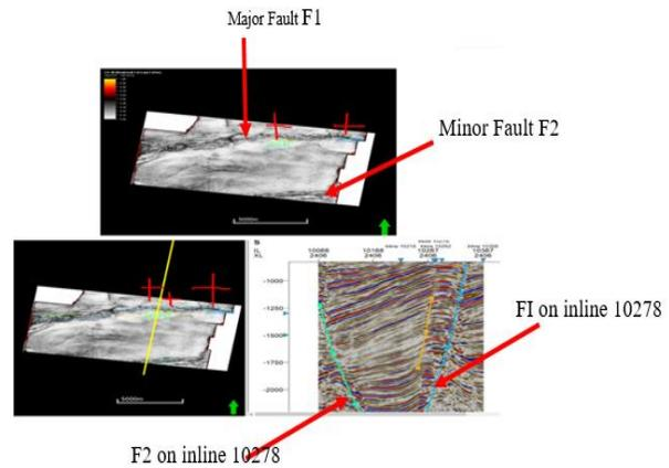
**Fig.s 10: Seismic section showing the NW-SE trending fault (F1 & F2) major fault that host hydrocarbon in Maboro-Field.**
