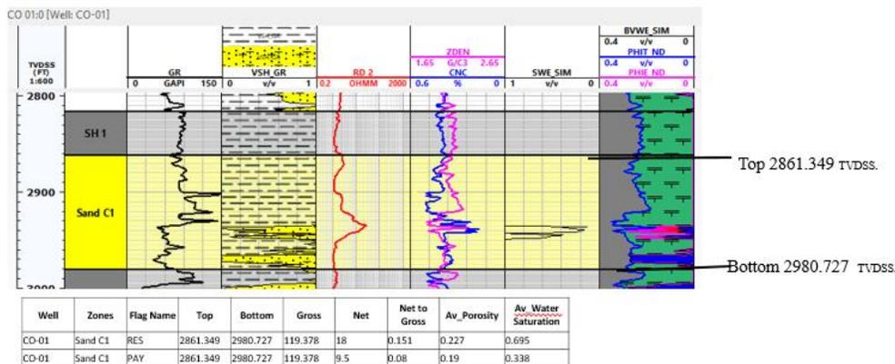
Fig. 8: The sand CO-01 C1 reservoir is a shaly sand with good resistivity value, poor porosity, moderate water saturation and the Neutron Density cross over indicates a small Gas. From this Fig. it is evident that the CO-01 C1 reservoir is highly compacted and can affect the productivity.
