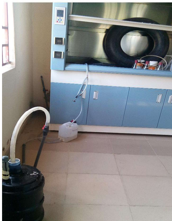
Fig. 1: Biogas production setup
