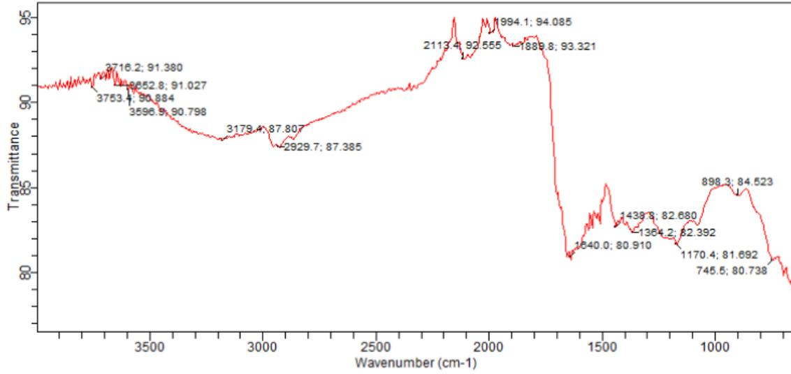
Fig. 3: FTIR of biochar after adsorption of Zn<sup>2+</sup>
