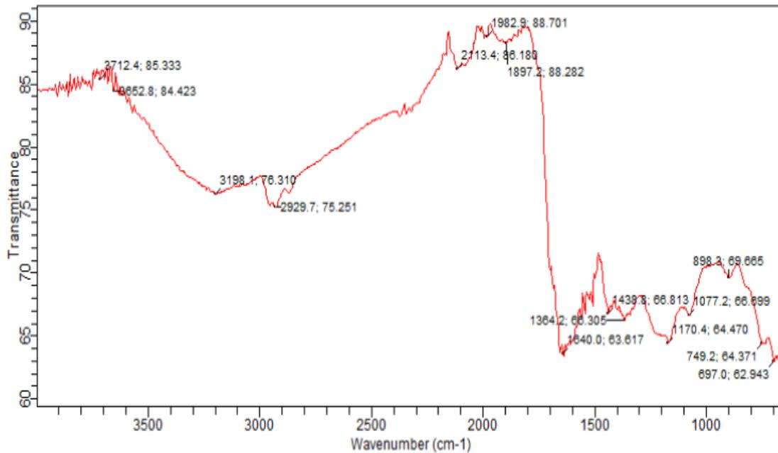
Fig. 2: FTIR of biochar after adsorption of  $Cd^{2+}$ .
