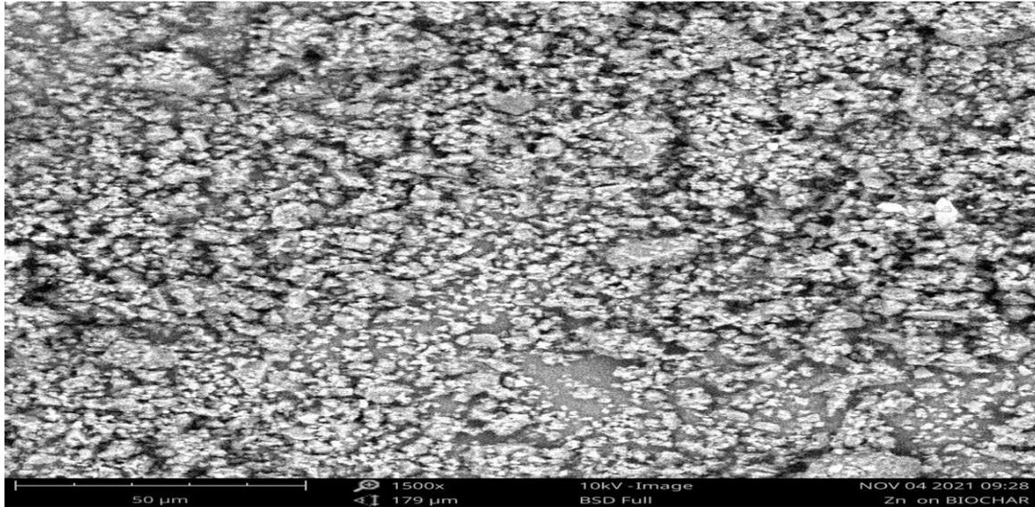
**Fig. 6: Scanning electron micrograph of biochar after adsorption of Zn<sup>2+</sup>. 3.1.2 Batch adsorption study**
