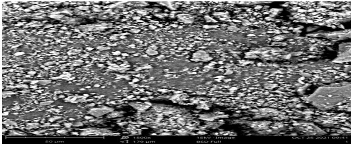
Fig. 4: Scanning electron micrograph of goat horn
