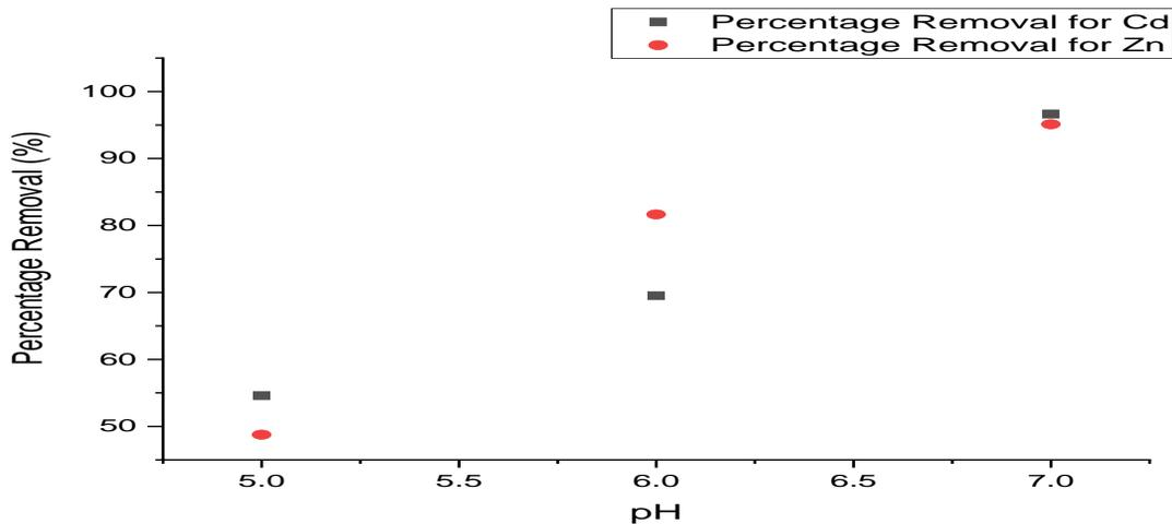
**Fig. 7: Effect of pH on percentage adsorption of Cd<sup>2+</sup> and Zn<sup>2+</sup> on biochar**
