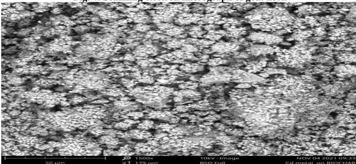
Fig. 5: Scanning electron micrograph of biochar after adsorption of Cd<sup>2+</sup>
