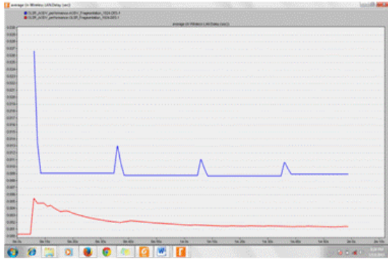
Fig. 7b: Delay comparison of 5 nodes scenario with fragmentation threshold at 1024 bytes
