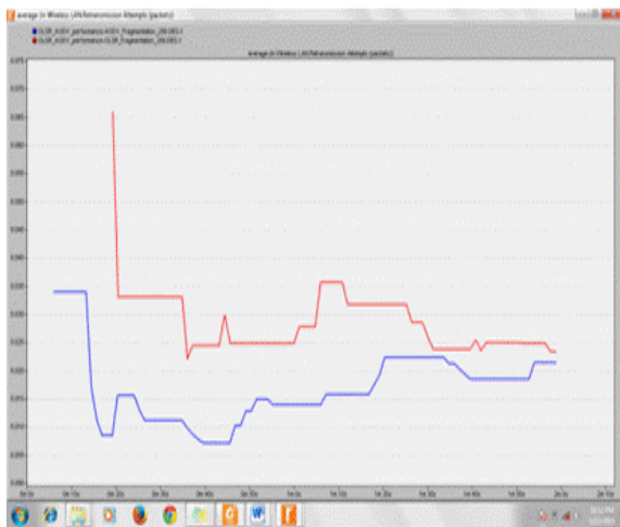
Fig. 9A: Transmission attempt comparison in 5 nodes scenario under fragmentation threshold of 256 bytes
