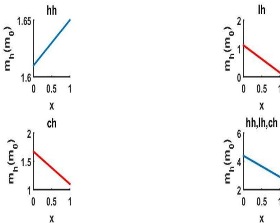
Fig.3: Hole effective mass ( $\perp$ ) as a function of composition  $x$
