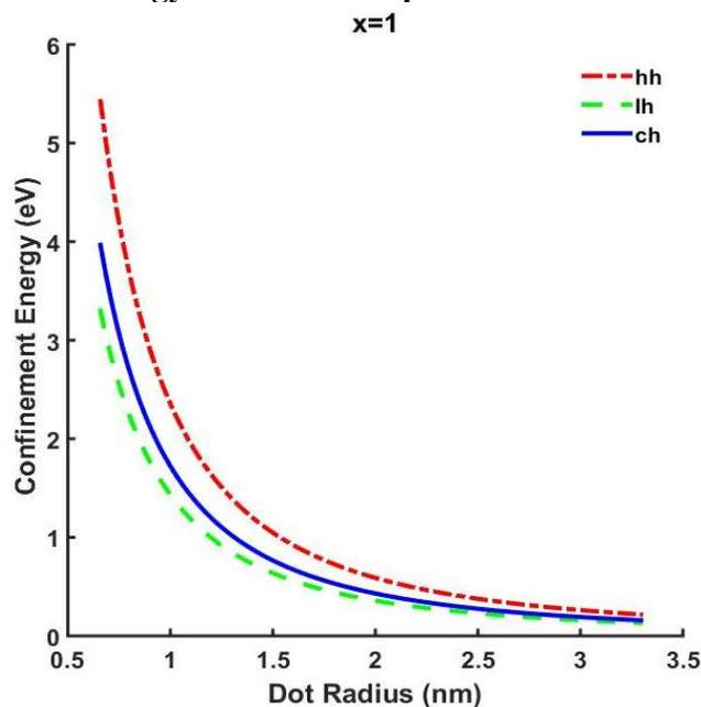
**Fig.7: Confinement energy at x=1 composition as a function of dot radius**
