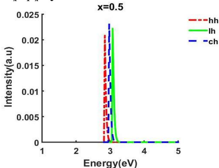
Fig.9: Emission intensity of hh, lh, chsubbands at 0.5 composition(x) as a function of photon energy in  $\alpha - \text{Ga}_x\text{In}_{1-x}\text{N}$  QD.
