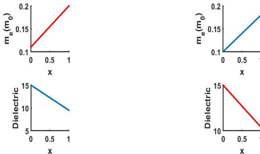
**Fig. 1: Variation of dielectric with composition,  $x$  for  $\alpha - Ga_xIn_{1-x}N$  nanostructure dots**
