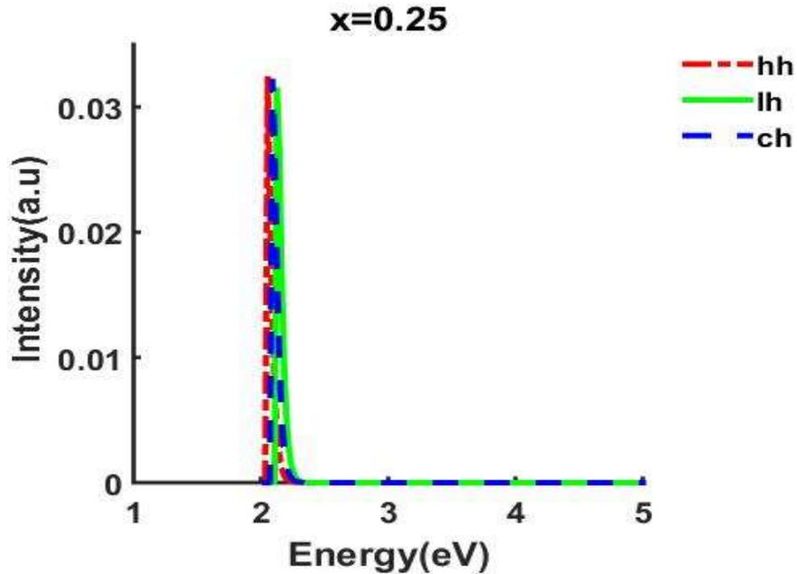
Fig.8: Emission intensity of hh, lh, chsubbands at 0.25 composition(x) as a function of photon energy in  $\alpha - \text{Ga}_x\text{In}_{1-x}\text{N}$  QD.
