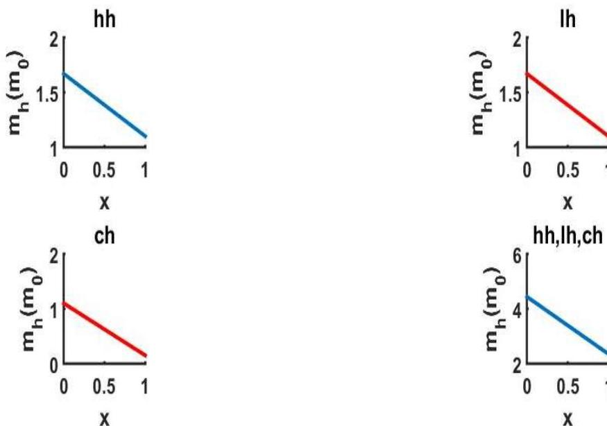
Fig.2: Hole effective mass ( $\parallel$ ) as a function of composition  $x$
