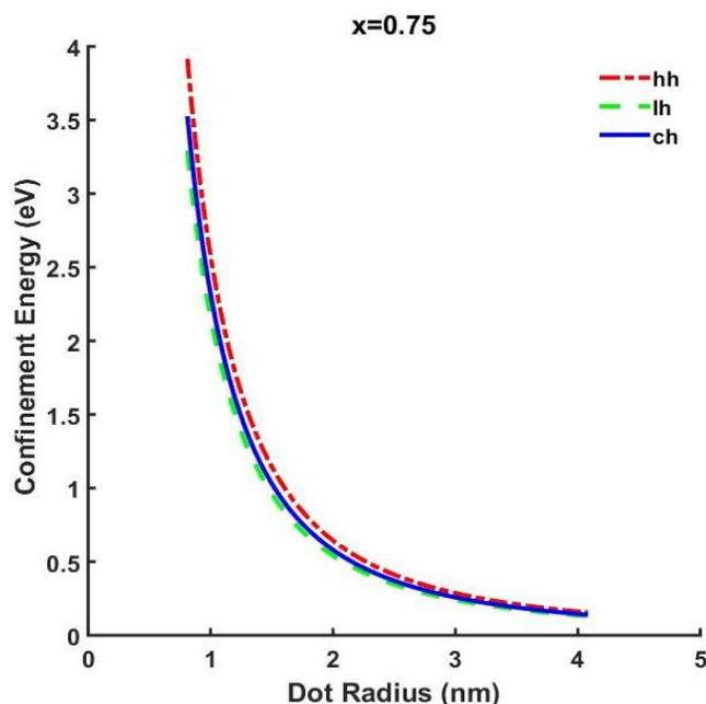
**Fig.6: Confinement energy at x=0.75 composition as a function of dot radius**
