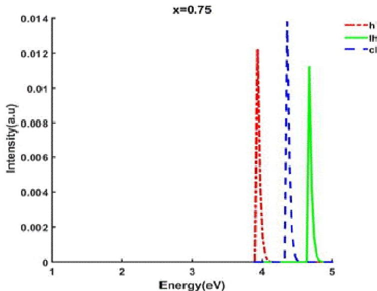
**Fig.10: Emission intensity of hh, lh, ch subbands at 0.75 composition(x) as a function of photon energy in  $\alpha - \text{Ga}_x\text{In}_{1-x}\text{N}$  QD**
