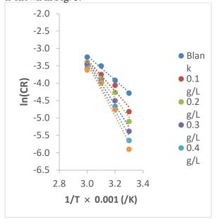
Fig. 5: Variation of ln(CR) with 1/T for the adsorption of ethanol extract of PT leaf on mild steel surface
