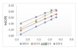
Fig. 7: Langmuir isotherm for adsorption of ethanol extract of PT on mild steel surface
