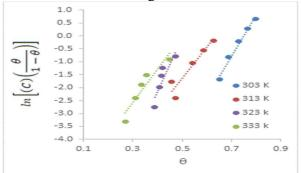
Fig. 8: Frumkim isotherm for adsorption of ethanol extract of PT leaf on mild steel surface
