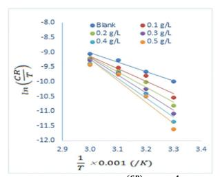
Fig. 6: Variation of  $ln\left(\frac{CR}{T}\right)$  with  $\frac{1}{T}$  for the adsorption of ethanol extract of PT leaf on mild streel surface
