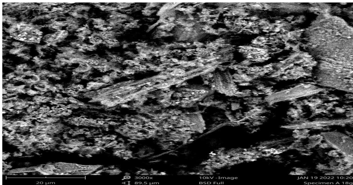
**Fig. 2 Scanning electron micrograph of H<sub>3</sub>PH<sub>4</sub> modified activated carbon**
