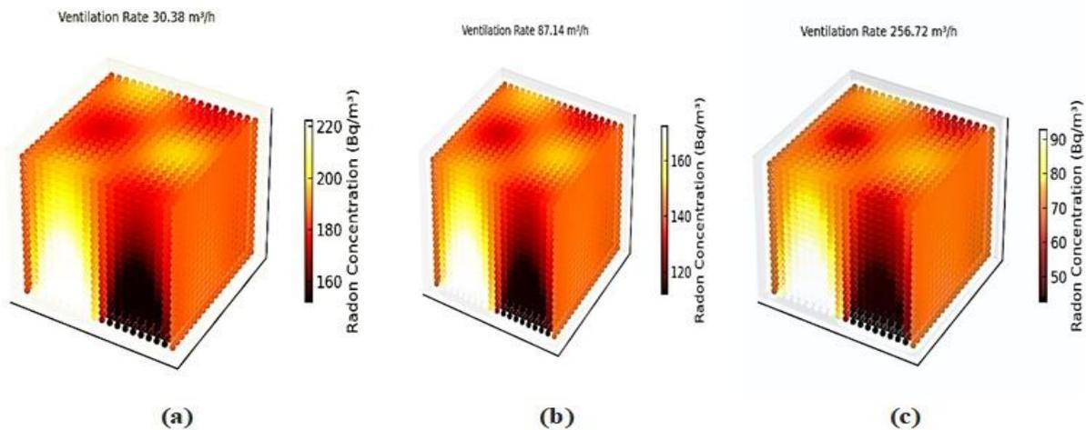
**Fig. 2: Modelled Radon gas concentrations at different ventilation rates 30.38, 87.14 and 256.72 m<sup>3</sup>/h using Ansys fluent 2025 R1 software**
