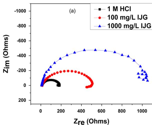
**Fig. 8: Nyquist plots for the inhibition of the corrosion of aluminium in 1 M HCl by 100 and 1000 mg/L concentrations of *Irvingia gabonensis* leaf extracts.**
