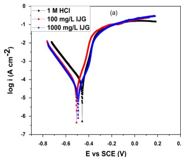
**Fig. 3: Potentiodynamic polarization plots for the inhibition of the corrosion of aluminium by leaf extract of *Irvingia gabonensis***
