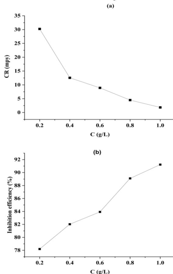
**Fig. 1: Variation of (a) corrosion rate of aluminium with concentration (b) inhibition efficiency of various concentrations of *Irvingia gabonensis* leaf extract with concentration at 303 K**
