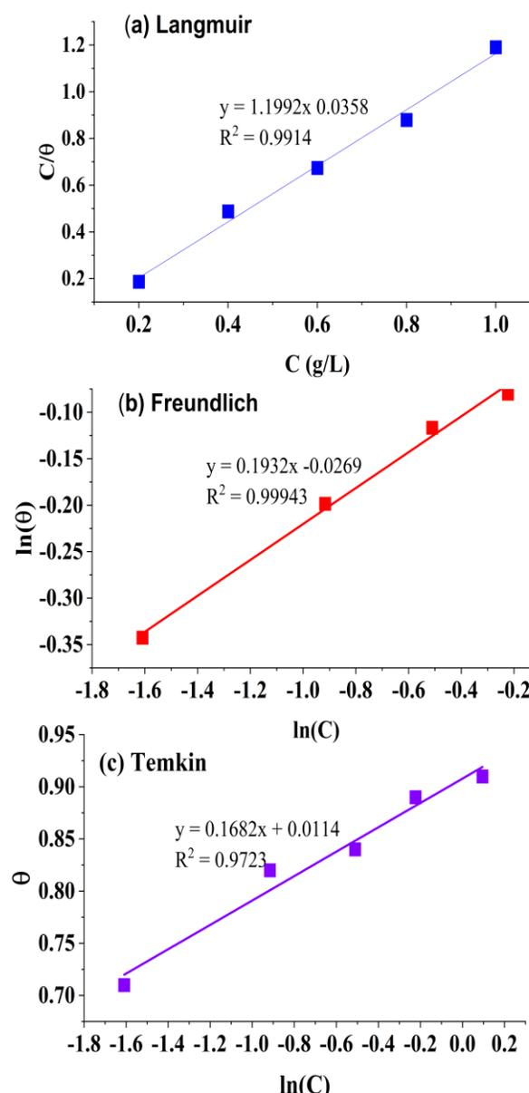
**Fig 5 Langmuir isotherm for adsorption of *irvingiagabonensis* on aluminum surface**
