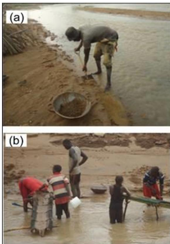
**Fig. 4. Artisanal mining in the study area with the use of rudimentary tools. (a) Artisanal miners panning for gold. (b) Shaking table used for the recovery of gold**
