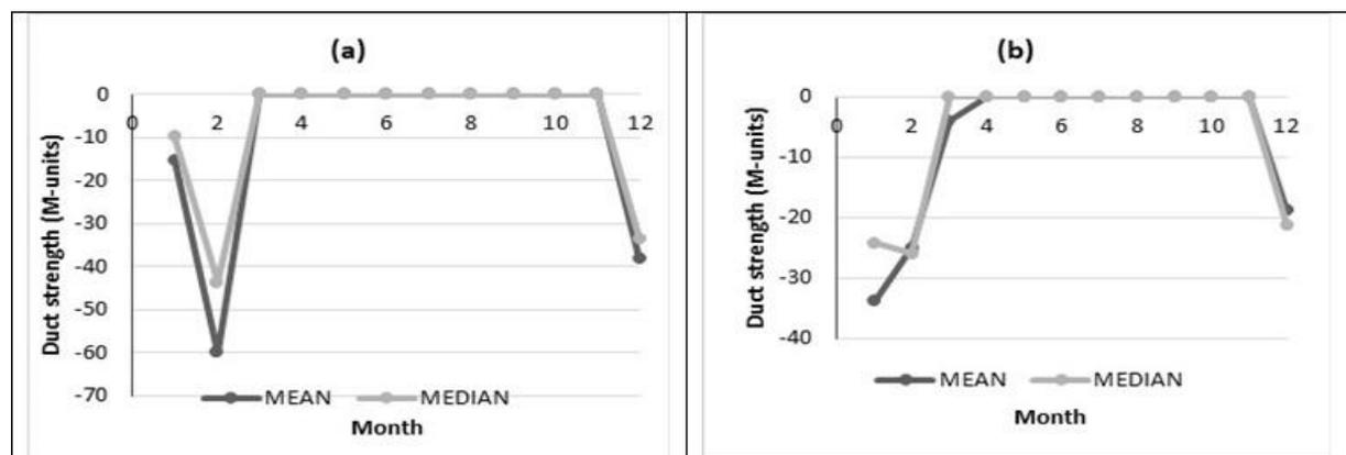
**Fig 11: Monthly variation of duct strength at 12:00 hour LT over (a) 100 m heights and (b) 300 m heights**
