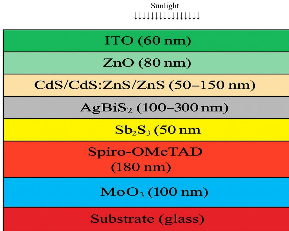
**Fig. 1: A diagrammatic configuration of the AgBiS<sub>2</sub> thin-film solar cells (ITO/ZnO/CdS/CdsZns/ZnS/AgBiS<sub>2</sub>/Sb<sub>2</sub>S<sub>3</sub>/Spiro-OMeTAD/MoO<sub>3</sub>)**
