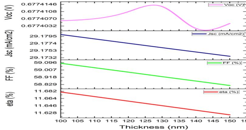
**Fig 2. Effect of MoO<sub>3</sub> hole transport layer (HTL) thickness on the photovoltaic (PV) performance**
