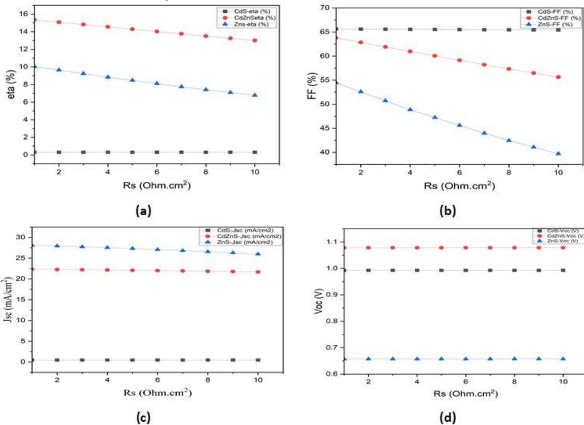
**Figs. 9a-d depict the effect of series resistance ( $R_s$ ) on device performance parameters, including  $\eta$  (%), FF (%), ( $J_{sc}$ ), and ( $V_{oc}$ ).**
