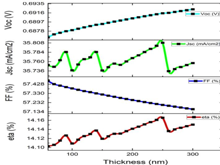
**Fig. 3** presents plots of the absorber thickness vs. the key photovoltaic parameters.
