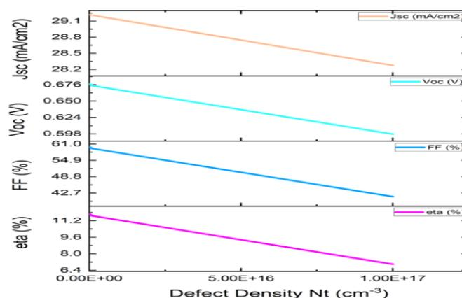
**Fig 4. Illustrate a plot of AgBiS<sub>2</sub> Absorber Defect Density vs Perovskite metrics:  $\eta$  (%), FF (%),  $J_{sc}$  and  $V_{oc}$**
