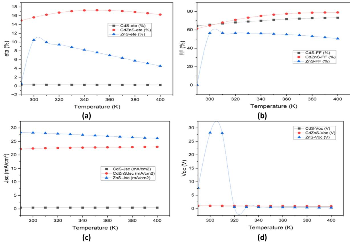
Fig. (7a)-(d) depict how Temperature impacts photovoltaic performance parameters
