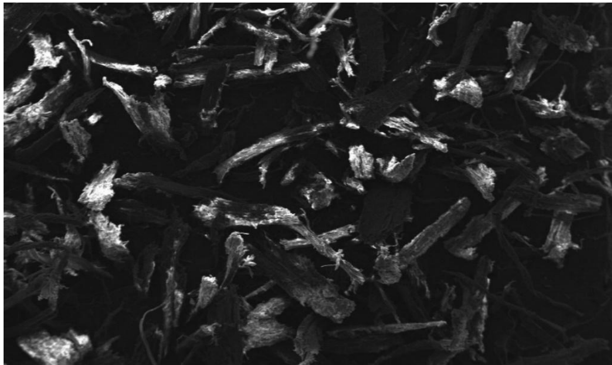
Fig. 2: Scanning electron micrograph of SiONPs synthesized from rice husk
