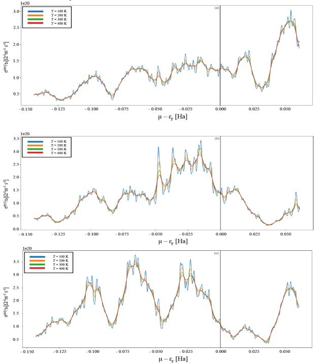
Fig. 5: Calculated Electric conductivity of MgS<sub>2</sub> for (a) xx component, (b) yy component and (c) zz component.
