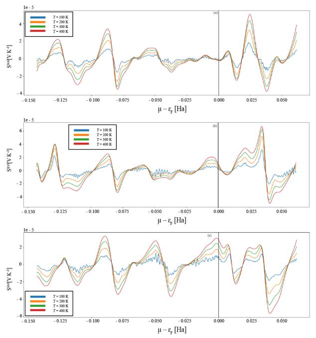
Fig. 4: Calculated Seebeck of MgS<sub>2</sub> for (a) xx component (b) yy component and (c) zz component
