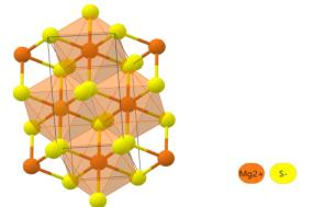
Fig. 1: Trigonal lattice structure of MgS<sub>2</sub> (Materials Project, n.d.)
