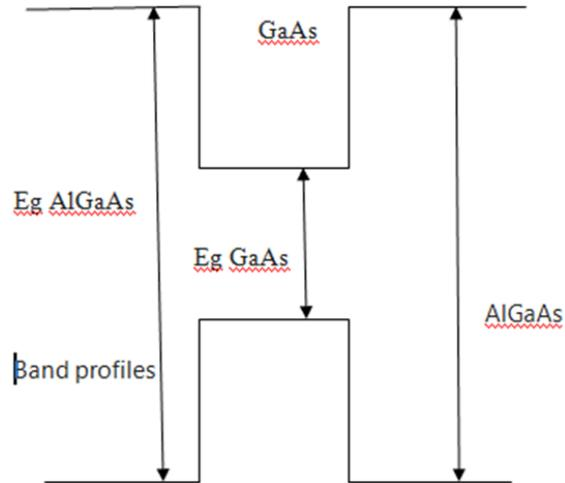
**Fig.1: diagram of quantum well using semiconductor**
