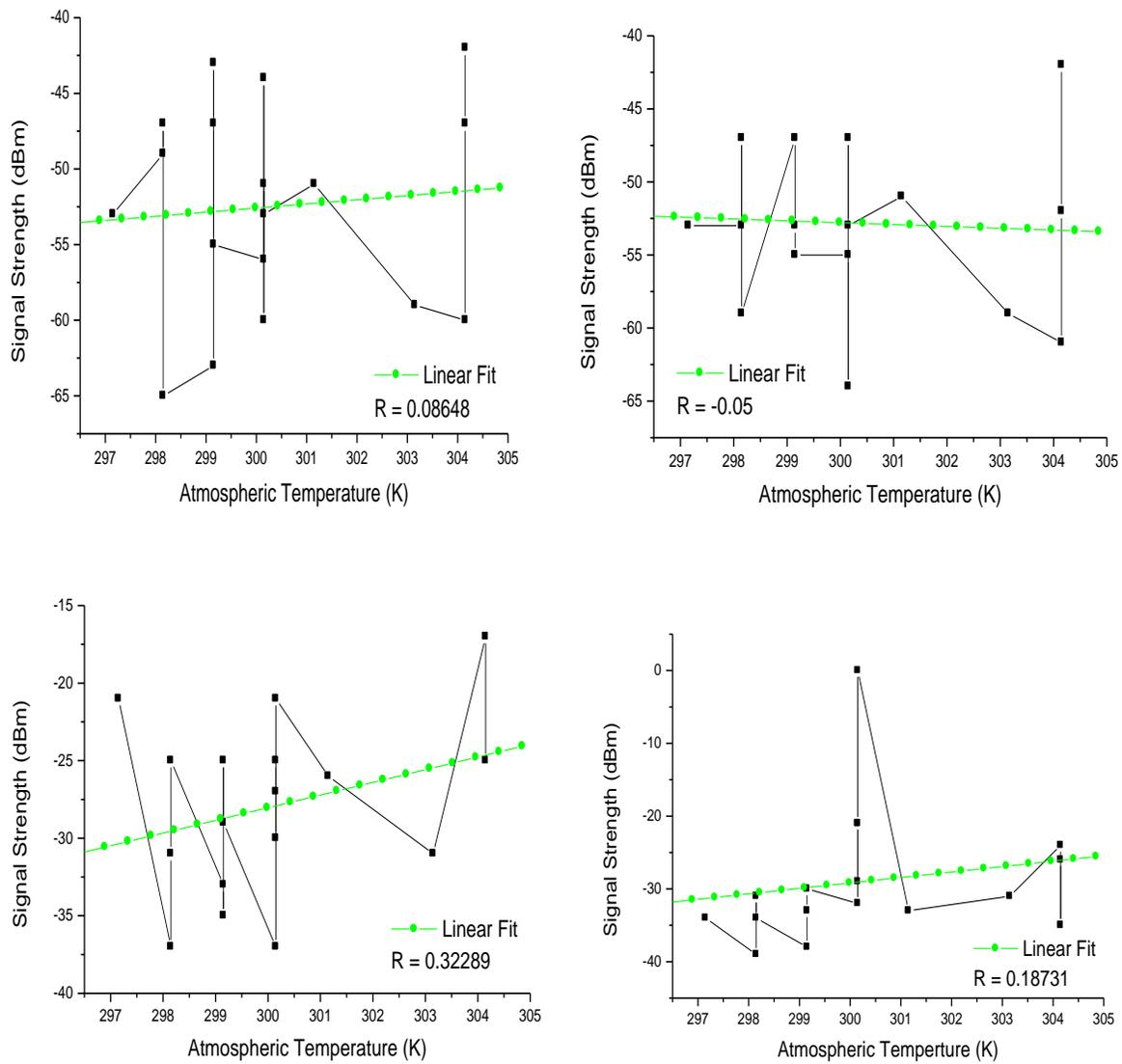
**Fig.1 Signal strength VS Atmospheric Temperature in Some Cells in Calabar**
