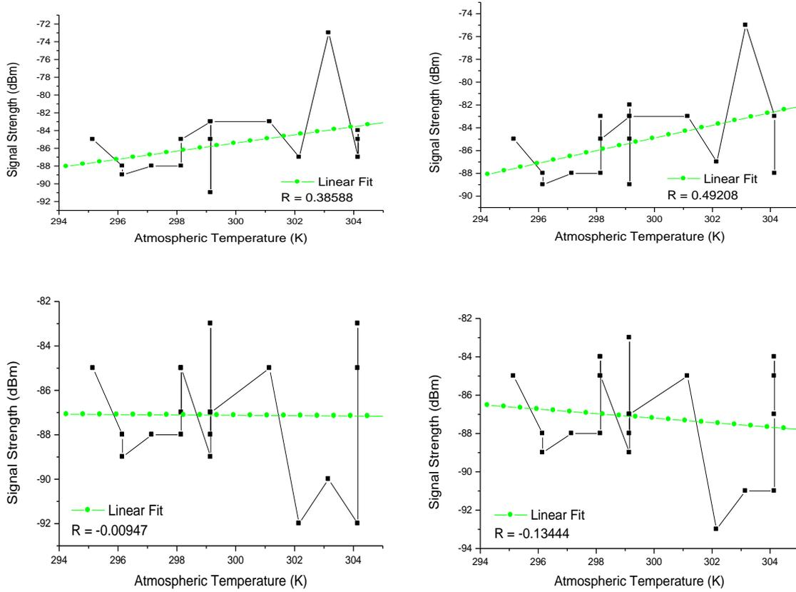
**Fig.4: Signal strength VS Atmospheric Temperature in Some Cells in Warri**
