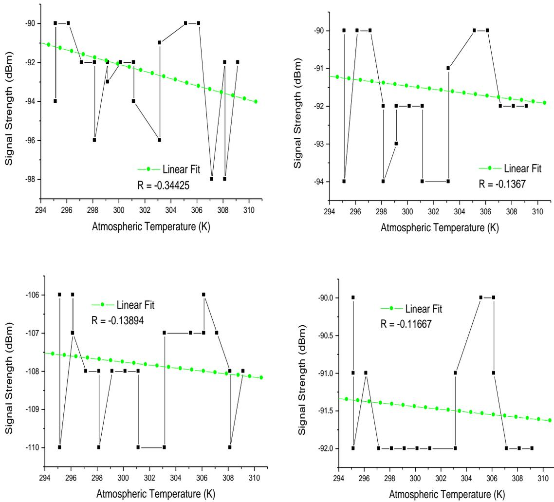
**Fig.2 Signal strength VS Atmospheric Temperature in Some Cells in Uyo**
