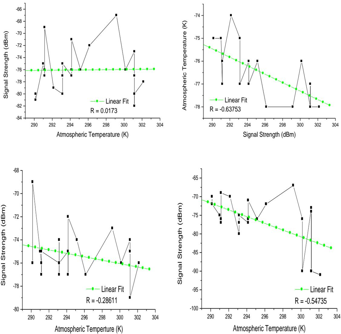
**Fig.3 Signal strength VS Atmospheric Temperature in Some Cells in Port Harcourt**
