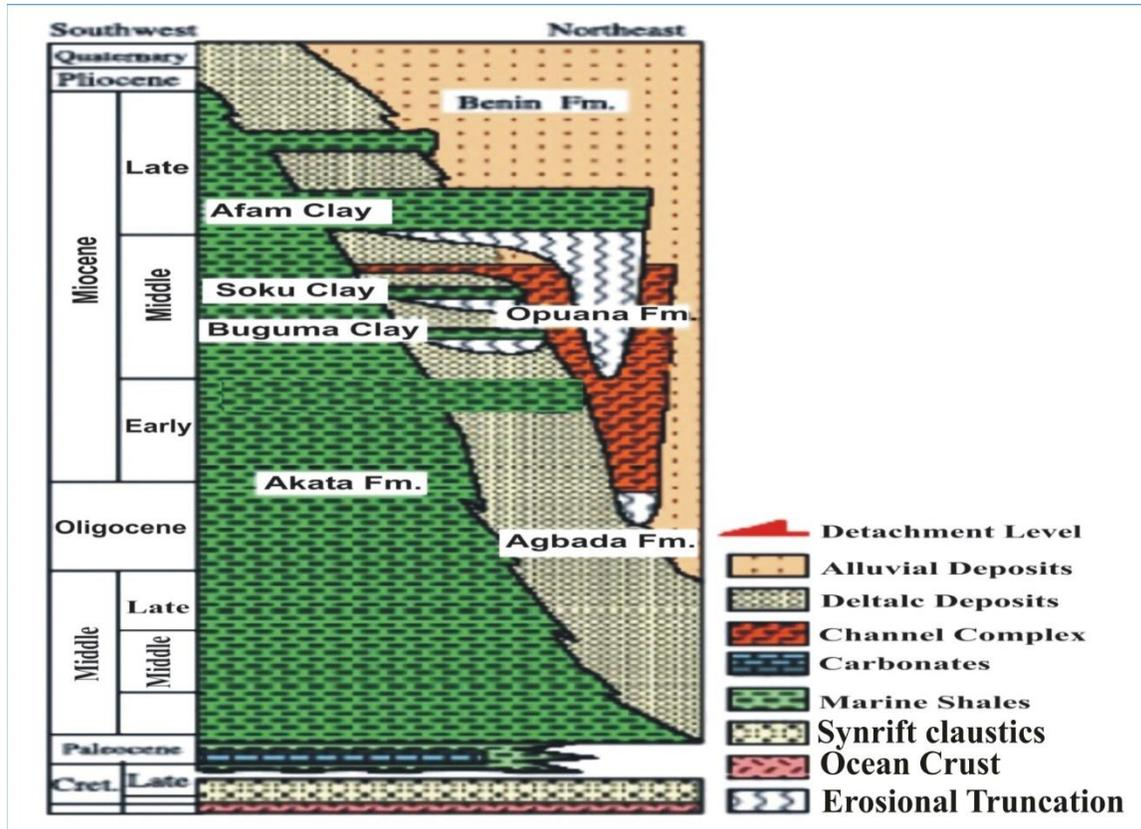
Fig. 2.: Stratigraphic Column showing three Formation of the Niger Delta Basin (Modified after Doust and Omatsola, 1990; Aigbadon et al., 2022).
