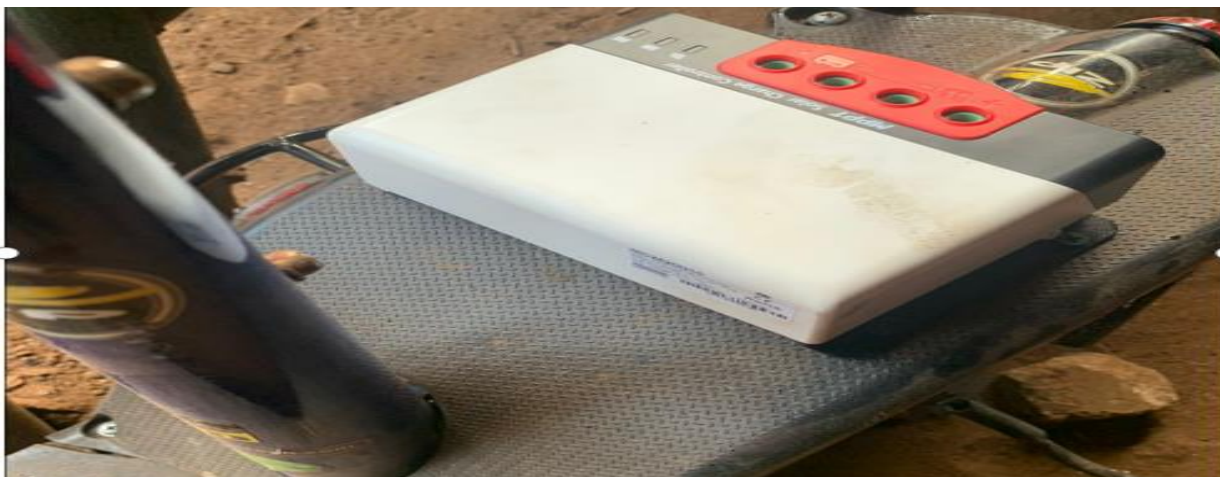
Fig. 3: Positioning of the charge controller on the scooter
