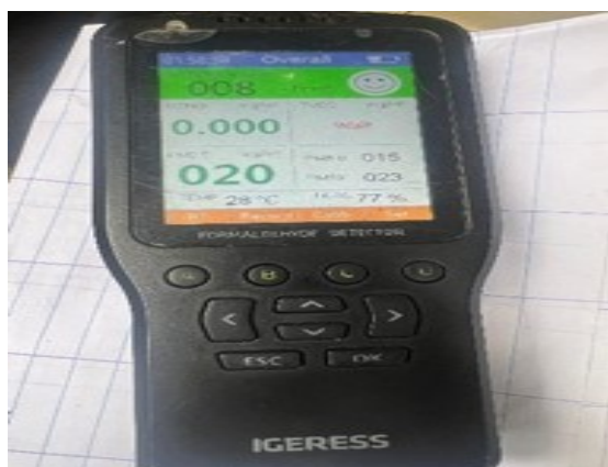
Fig. 1: Igeress formaldehyde detector (Air monitor)
