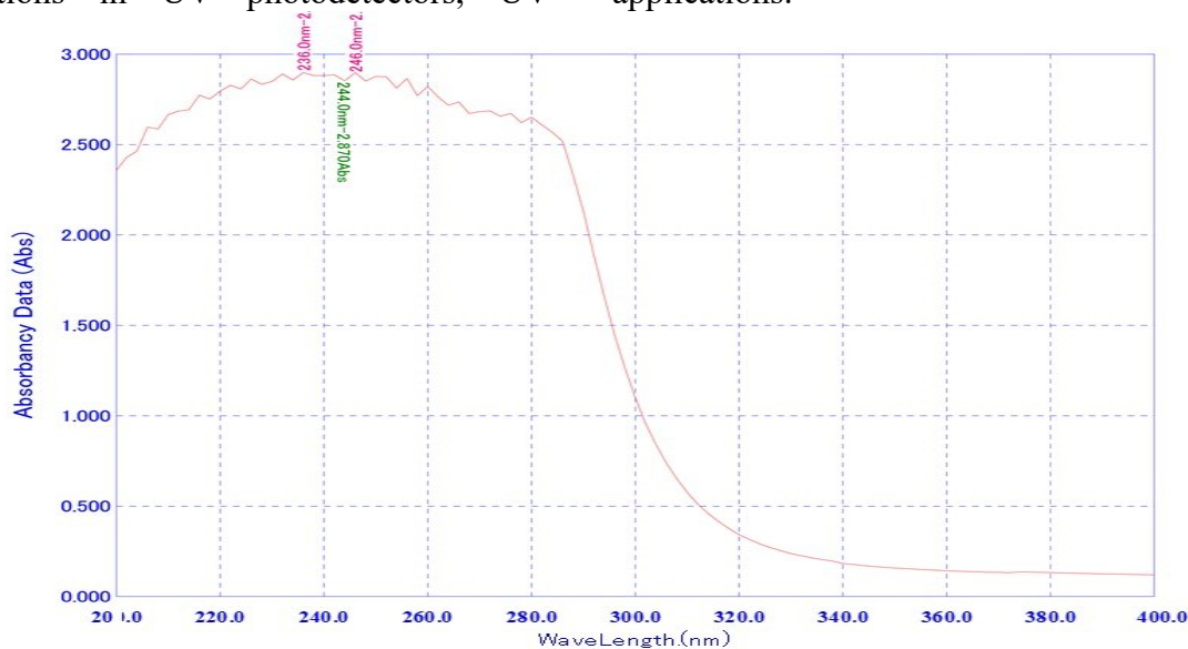
Fig. 1: UV visible spectrum of silicon quantum dots produced from waste coconut shell
