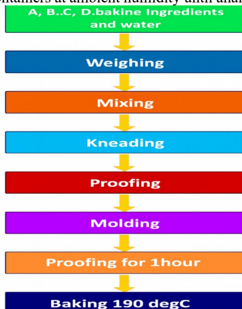
Fig. 1: Raw materials and composite snack-making flowchart
