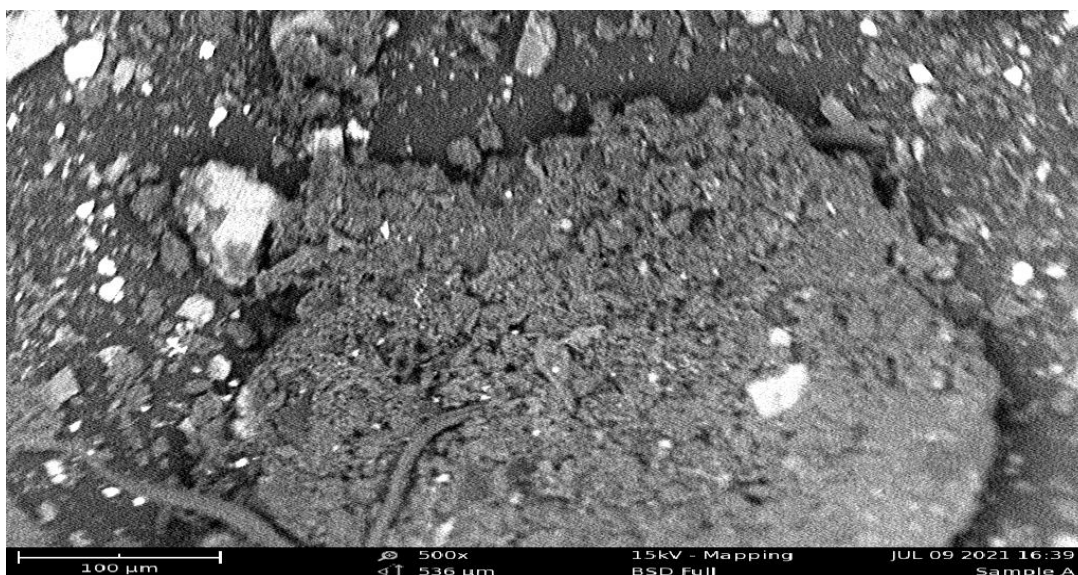
Fig 5: Zoom SEM image of aluminium oxide nanoparticles
